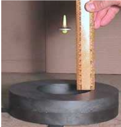
Fig1: The Levitron top levitating above its permanent magnet base.
