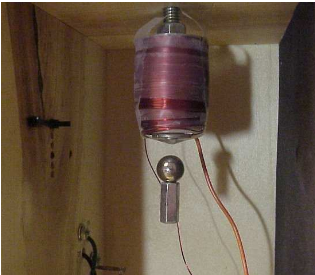
Fig6: Picture showing a magnetic suspension system in action.
