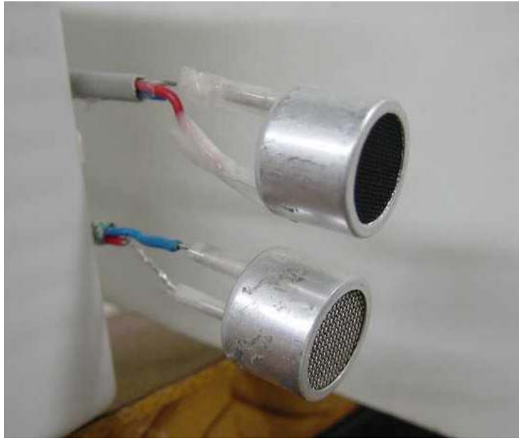
Figure 4.23: Piezoelectric 40 kHz transmitter and receiver transducers.
