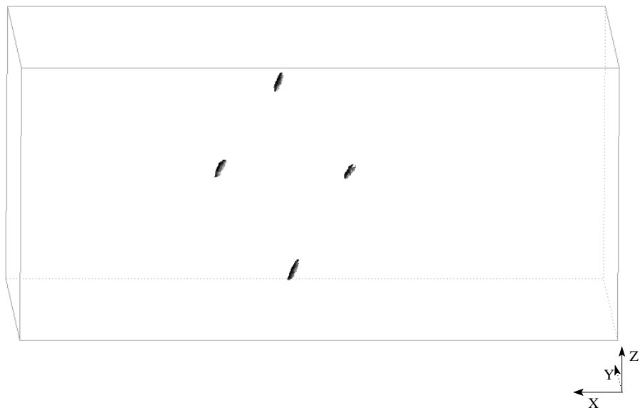
Figure 4.43: Reconstructed 3-D image from two focused magnitude sonar images taken from different view angles in a water tank.
