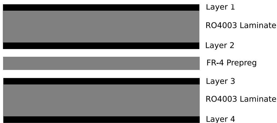
Figure 2.16: Non-standard stackup used for the board
