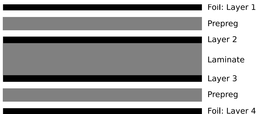
Figure 2.15: Standard stackup for four layer PCBs
